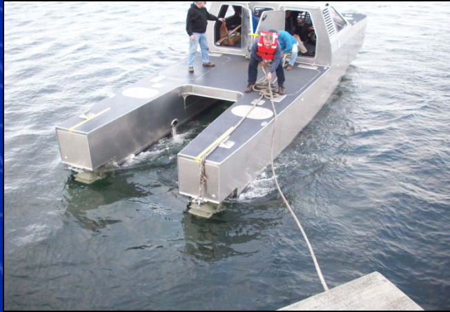
Small Tactical Craft Bollard Thrust Test North American Marine Jet Nomera 800 with "C" Impeller Port Angeles, Washington September 5, 2008 4:14 PM
